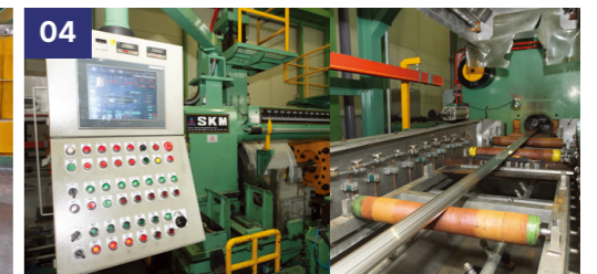
Extrusion(1,800 Ton / 7 inch) 2 line
